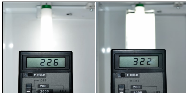
Intensity Reading of T8 Lamp with KOJIN Nano Reflector
